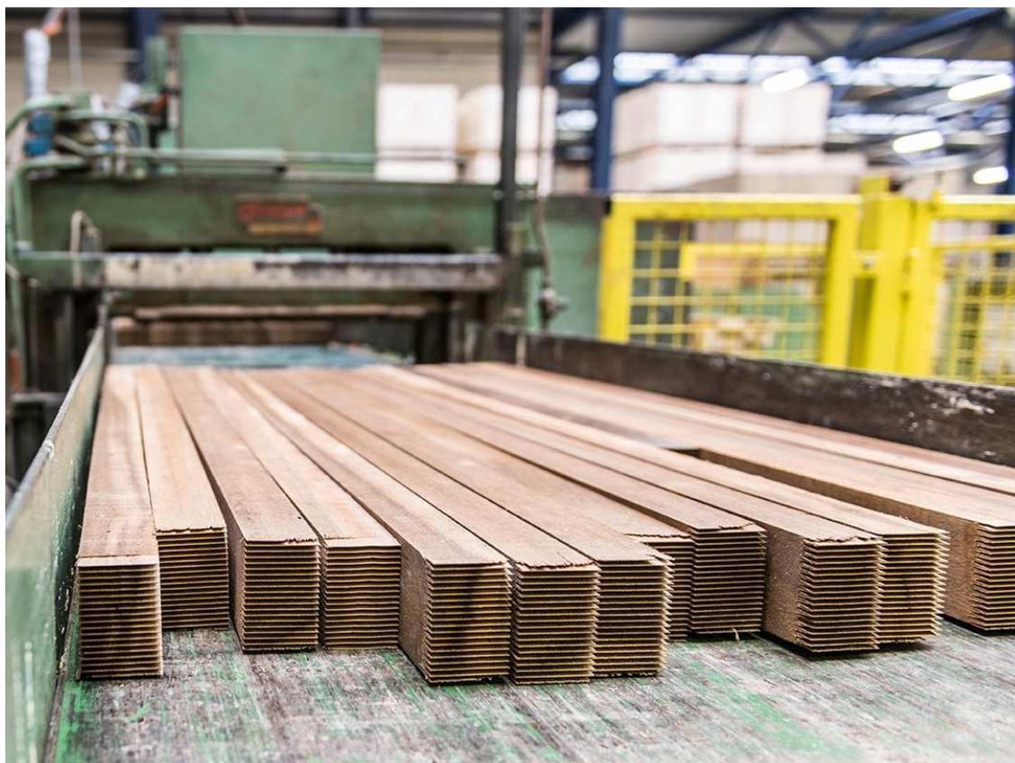
Picture 1: Shorts ready for the GluGreen finger-joint process. Photo: GluGreen BV
